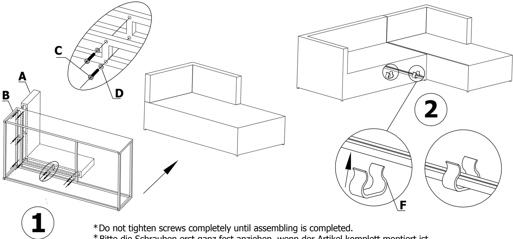
\* Do not tighten screws completely until assembling is completed.
